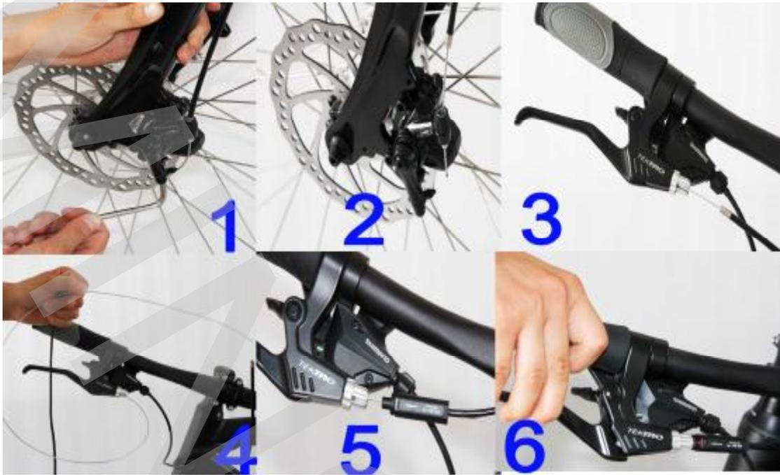
**5. Install Brake Sensor on the middle of brake line**
